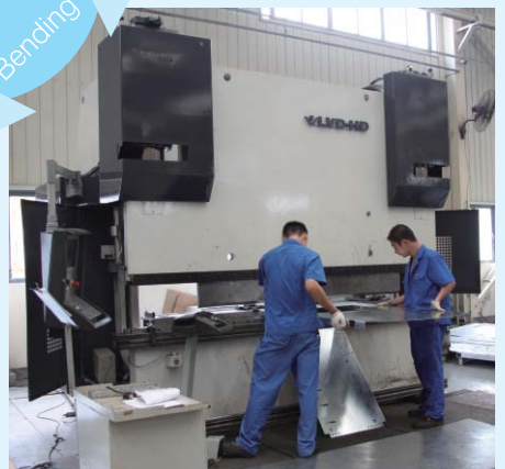
▲ PPEB220-30-5 CNC bending machine
